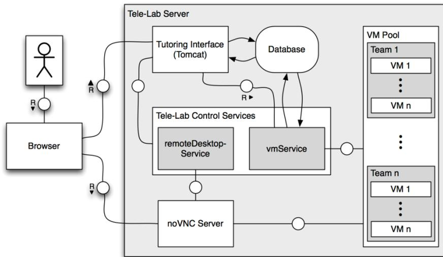
**Fig. 2: Architecture of the Tele-Lab Platform**
